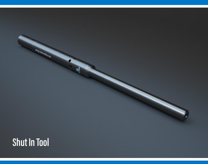
The Omega Shut In Tool is a single shot battery driven device which has been designed for basic well testing situations when a flowing well is shut in downhole and the resulting pressure build up is monitored by memory gauges.
