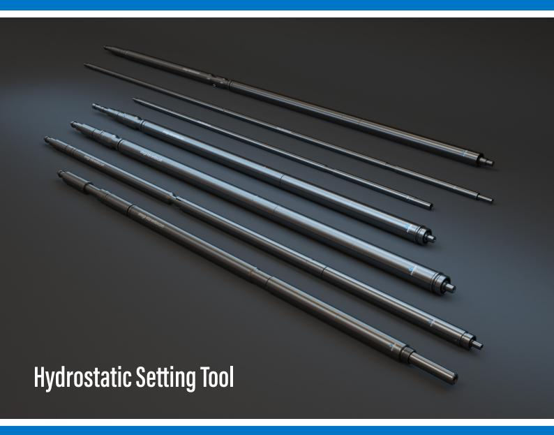
The Omega Hydrostatic Setting Tool (HST) provides the industry with a highly reliable, non-pyrotechnic setting device used for the installation of downhole tools such as bridge plugs, high expansion gauge hangers, and straddles.
