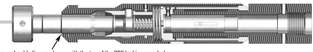
Bottom groove should align as shown with the top of the RRS locking mandrel.
