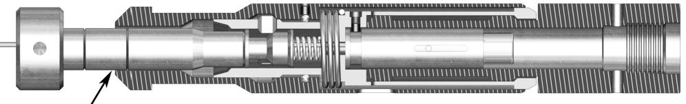
The top of the locking mandrel is in between the two grooves.
