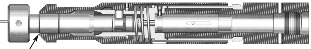
Once stroked the top groove should align as shown with the top of the locking mandrel. After the function check the rope socket Can then be re-set to the locked position by removing the trigger gauge and sliding the locking mandrel downwards.
